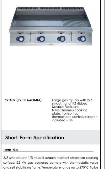
and self stabilizing flame. Temperature range up to 270°C. To be installed on open base installations, bridging supports or cantilever systems. Removable drawers below the cooking surface for the collection of grease and fat. Body and work top of unit entirely in stainless steel with Scotch Brite finish. Extra strength work top in heavy duty 2 mm stainless steel. Rightangled side edges to allow flush-fitting junction between units.
